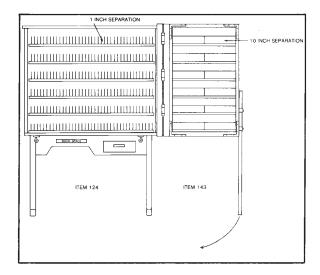
221.33 This case, with wing, shows how the separations may be arranged when more than 6 rows of separations are needed for letters. When so arranged, all are within reach and mail will not have to be rehandled.
